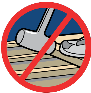
T&G edges are designed to self-space.
